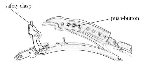
Lift safety clasp and press both push-buttons to open closure
